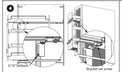
Pull top front mounting bracket into position on side of face frame (or cabinet) allowing for a 3/16" setback (shown left above). Firmly secure with one (1) #8 x 5/8" Pan Head Wood Screw (**D**). Make sure gap between unit and side of face frame is equal from top to bottom. Adjust accordingly and then securely tighten bracket set screw (shown right above).
