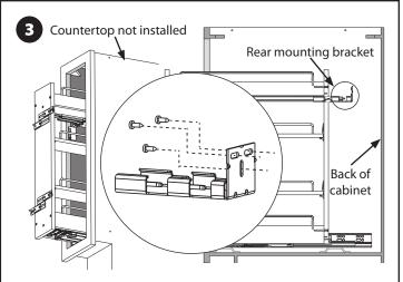
If countertop is not installed, pull organizer partially out to gain access to rear bracket from top of cabinet and install three (3) #8 x 5/8" Pan Head Wood Screws **(D)** provided in slots.
