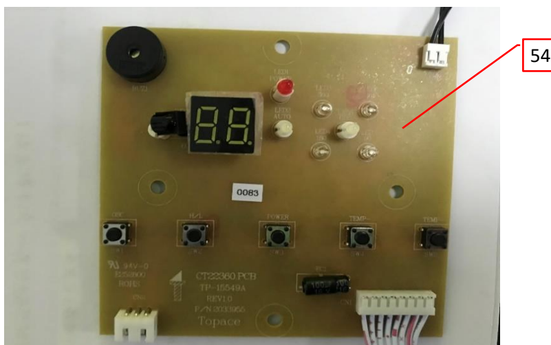
Photo 6.2 - Display PCB, Shenzhen Topace Technology CO Ltd, 2033955
