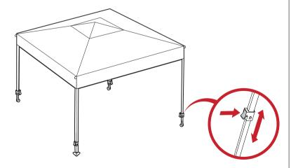
Secure with four part C ropes and eight part D stakes.
