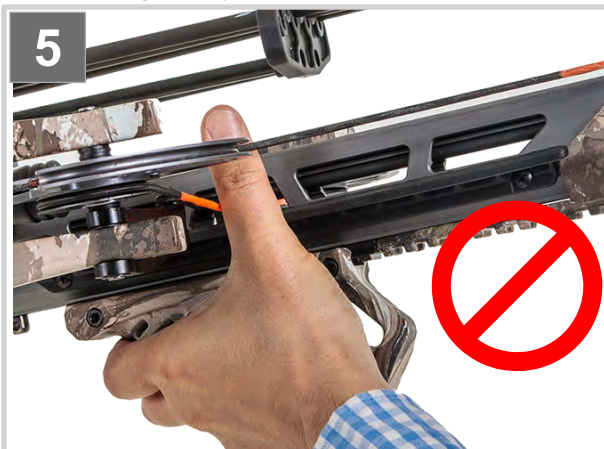
Pic 5. Improper Hand Position – with your fore-grip positioned as shown you will have a severed hand or finger amputation
