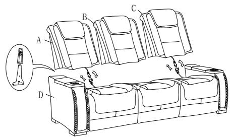
Step 2 Connect the power supply (E) to the wire on seat (D). Lastly, connect the lamp plug (F) to the wire on the middle backrest (B).
