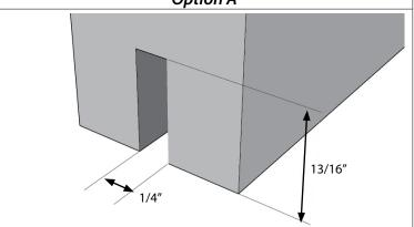
Mortise a 1/4" wide x 13/16" deep groove in the center bottom of the door to use with the floor-mounted door guide. This will prevent the door from swinging in and out and ensure smooth travel side-to-side.
