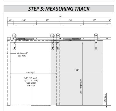
When installing into drywall, a piece of solid wood blocking is required to be mounted inside or outside of the wall before proceeding with the track installation. Position the solid wood blocking with track by measuring up from the door height (DH) + 1-11/16" to the center of the track. This allows a 3/8" - 1/2" gap at the bottom. For outside wall blocking, ensure it is level and leave a minimum of 2" from the end of the blocking to the side of the opening.
