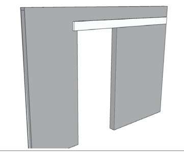
**SURFACE MOUNTED:** The track can be installed using surface wood blocking mounted to the structural surface of a wall using mounting screws into studs. Use a stud finder where necessary to locate studs and safely secure.
