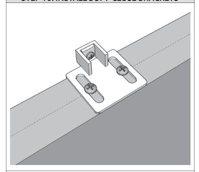
After door stops are adjusted, measure and mark the center of the door. Position the Soft-close Brackets to engage the Soft-close guide when it opens and closes. Mount and adjust the Soft-close Brackets using the screws provided.
