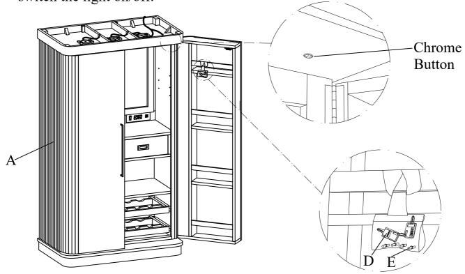
Open the other door of the Wine Cabinet (A). Insert the Shelf Pin (E) into the pre-drilled holes of the Wine Cabinet (A) and place the Shelf Frame (B) inside. Then, place the Glass (C) onto the Shelf Frame (B).
