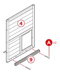
Attach a part 9 window frame to part 3 right side with two part A screws.
