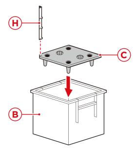
Insert the part H irrigation slot into the part C inner layer. Place the inner layer on the part B liner.
