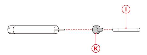
Insert the part I glass tube into the part K plug. Insert the plug/glass tube into the water pipe, making sure that the water indicator slides through the plug and can be seen in the glass tube.
