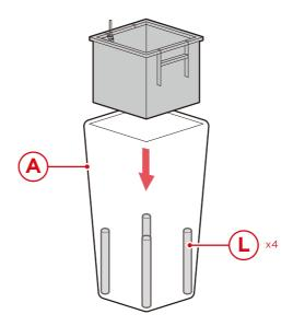
Place four part L inner legs into the part A planter. Place the liner onto the inner legs.
