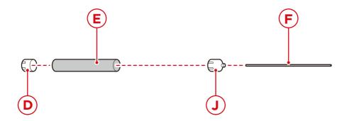
Slide the part E water pipe into the part D stopper. Insert the part F water indicator into the part J irrigation mechanism. Insert the water indicator/irrigation mechanism into the water pipe.
