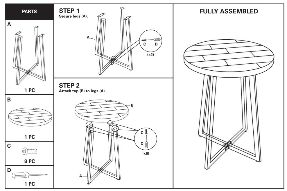
NOTE: FEET ON BOTTOM OF LEGS (A) ARE ADJUSTABLE FOR LEVELING.
