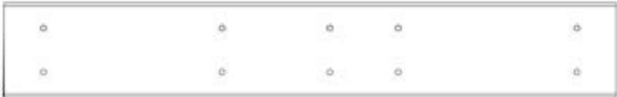
OG03 FLOOR JOIST - W4L22368 (x1) 1 3/16"x3 3/8"x21 7/8" (30x86x556)
