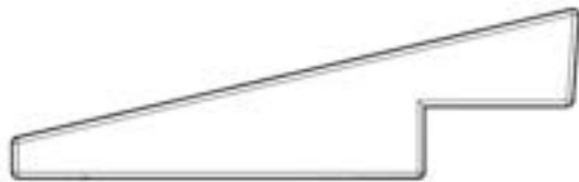
W03 ANGLE BRACE - W4L22911 (x2) 1 15/16"x3 3/8"x11 1/4" (50x86x285)
