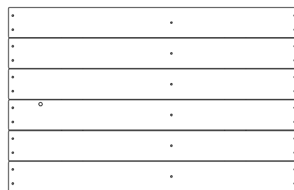
HH5 | FLOOR PANEL - W2A03076 (x1) | 1 1/4"x20 9/16"x32 7/16" (32x522x824)
