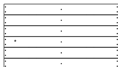
HH2 | FLOOR PANEL - W2A03080 (x1) | 36 3/8"x1 1/4"x20 9/16" (924x32x522)
