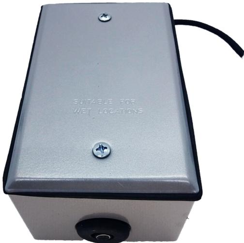
The SS-705 is an outdoor rated mic level microphone with an omni-directional pickup radius of approximately 12 feet. Housed in a weather resistant enclosure, the SS-705 is suitable for outdoor applications. The SS-705 does not require external power and is compatible with select IP cameras featuring a mic level audio input. The microphone includes 40 feet of cable with a 3.5mm plug. The cable may be threaded through either the top or rear of the enclosure.
