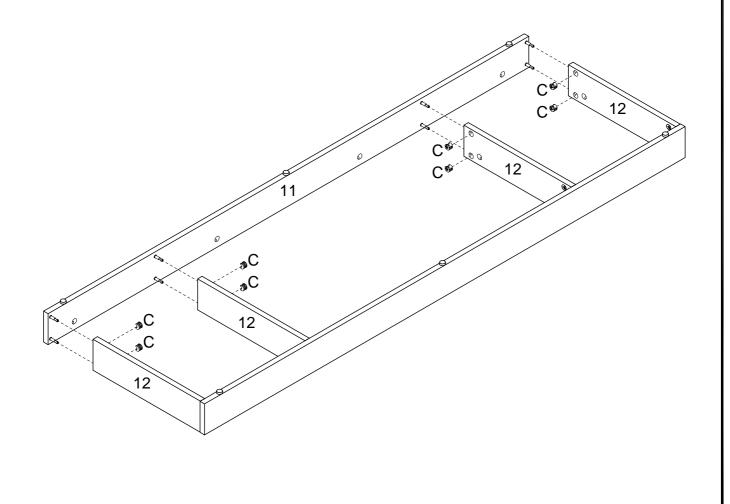
Place the plinth base you just built on the Bottom Frame (2) aligning with the cam bolts and secure with cam locks (C).
