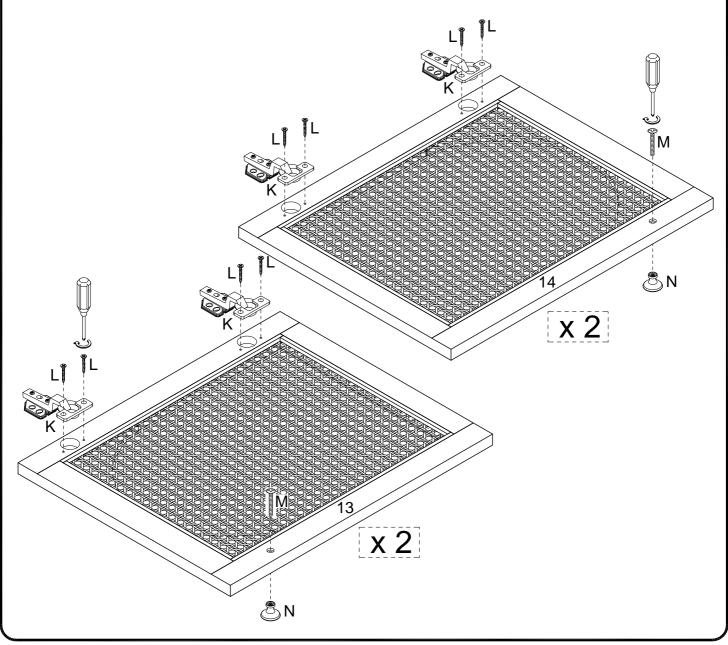
Secure the Left Door (13) to the case using screws (L).
