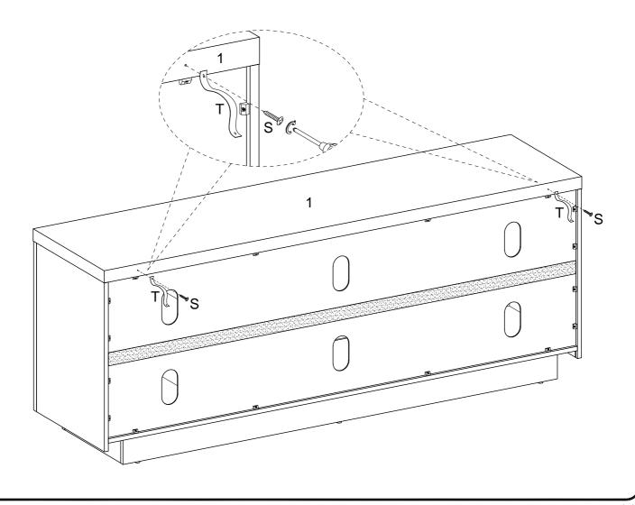
Attach the other end of the plastic strap (T) to your wall with the wall anchor (U) and screw (R). No tipping over here safe and secure!
