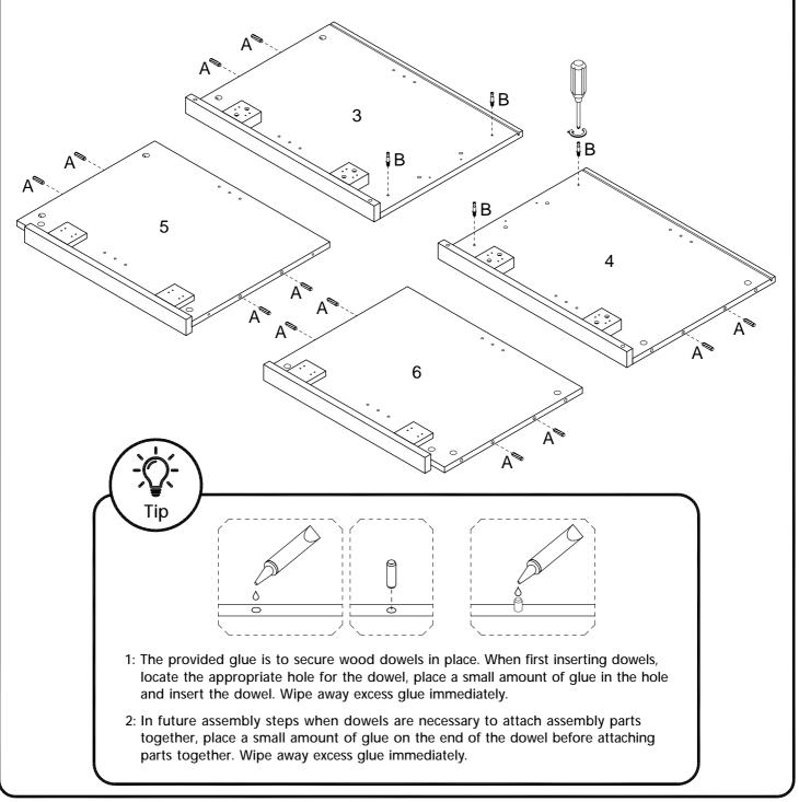
Insert those dowels (A) into the Bottom Frame (2) and the Top Rail (7).
