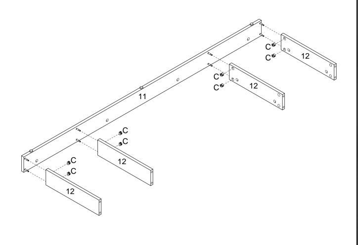
Attach the other Long Apron (11) to the Short Aprons (12) again with cam bolts (C). Plinth base is built!
