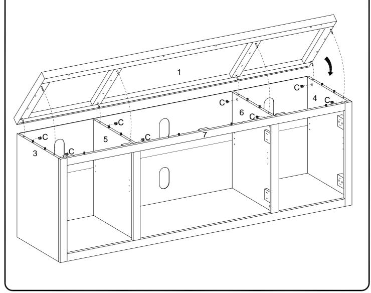
Carefully turn the whole thing onto the Top Panel (1). Screw in cam bolts (B) to the Bottom Frame (2) and screws (F) into the Top Rail (7).
