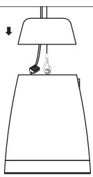
6. Plug the connected screw-terminal connector into jack on rear of speaker. Cut off any excess cable. Then close the magnetic back cover once done.
