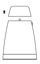
2. Lift the magnetic back cover off the speaker.
