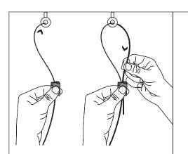
1. Pass the end of the cable through one hole of the gripple, then over the mounting structure, then through the other hole of the gripple.
