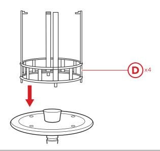
Attach the part 1 roof bracket to the roof supports.
