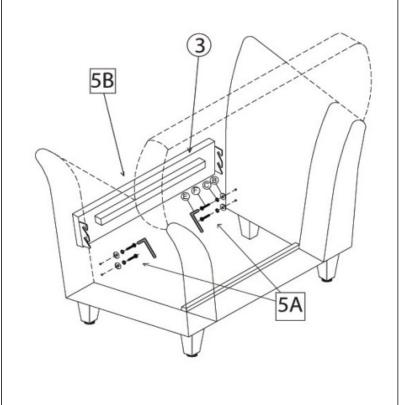
STEP 6:  $_{6A: \, Secure \, \, the \, Seat \, Panel \, to \, the \, chair \, frame \, using \, the \, screw \, "D"}$ into pre-drilled holes
