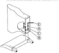
STEP 4: Repeat above steps for right side facing arm assembly NOTE:DO NOT OVER TIGHTEN BOLTS FOR EASY
