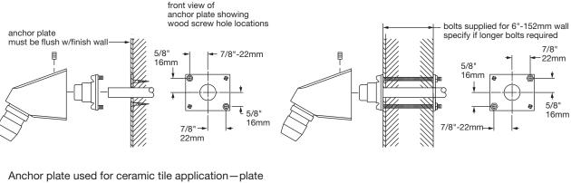
Anchor plate used for ceramic tile application—plate screws to wall and tile is applied up to sides of plate. Mounting bracket is mounted on finished wall with machine screws into anchor plate
