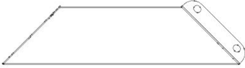
C02 CORBEL ASSEMBLY - A4M03526 (x1) 21 13/16"x5 1/4"x2 3/4" (70x134x553.5)
