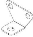
J7 RAFTER BRACKET - A4M03802 (x4) 3 5/8"x2 3/16"x2" (50x55x92)
