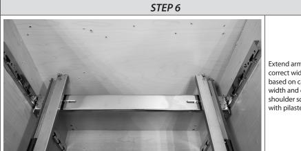
Extend arms to correct width based on cabinet width and connect shoulder screws with pilaster poles
