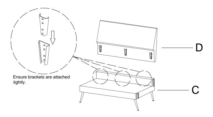
Connect Chaise Seat Frame (E) & Loveseat Seat Frame (C) by using brackets as drawing below.
