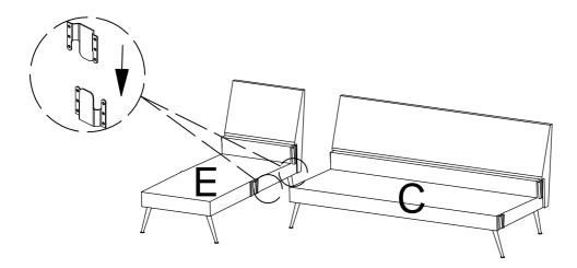
Attach Side Arm-RSF (A) & Side Arm-LSF (B) to Loveseat Seat Frame (C) & Chaise Seat Frame (E) by using brackets as drawing below.
