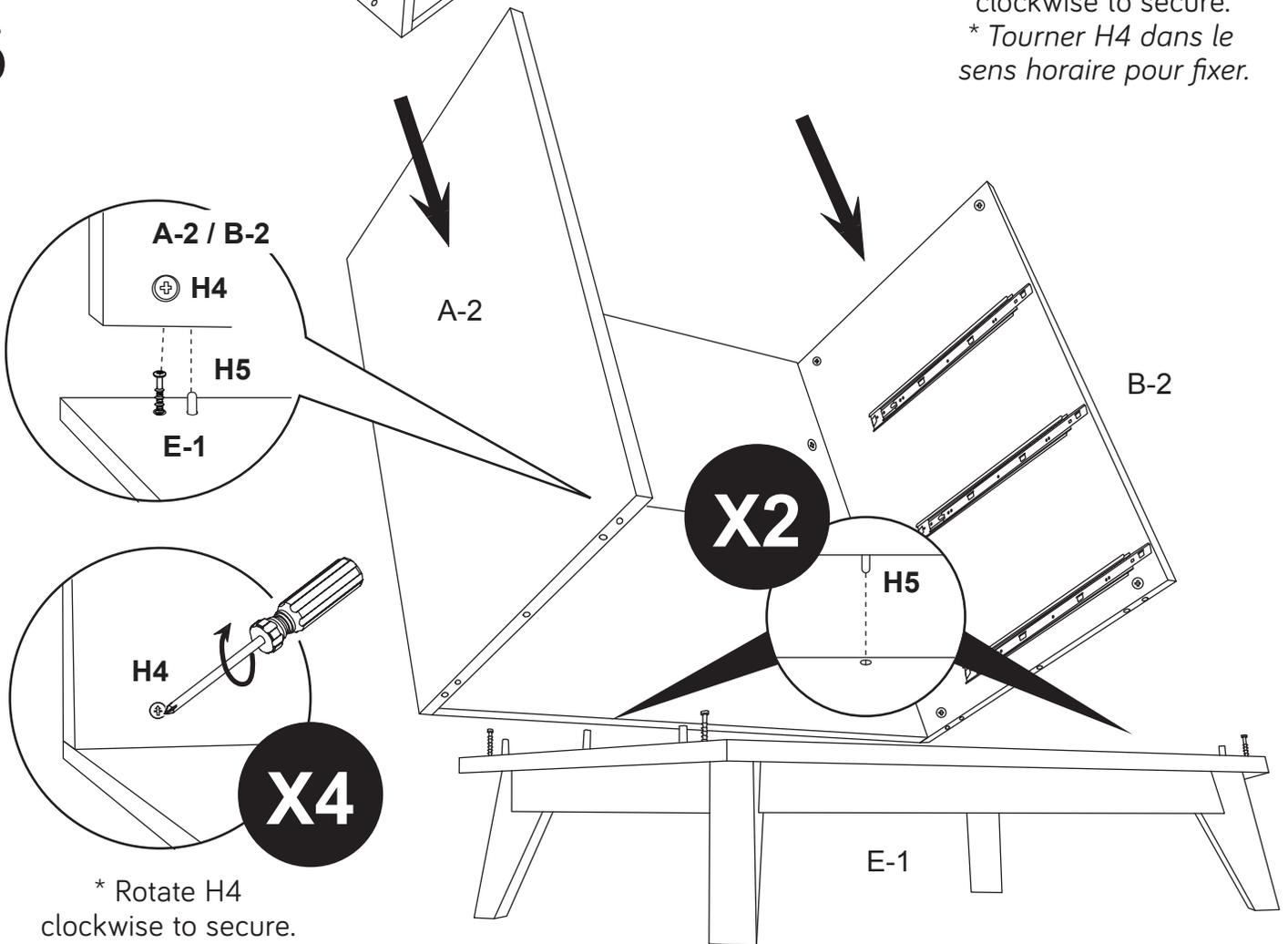
\* Rotate H4 clockwise to secure.
