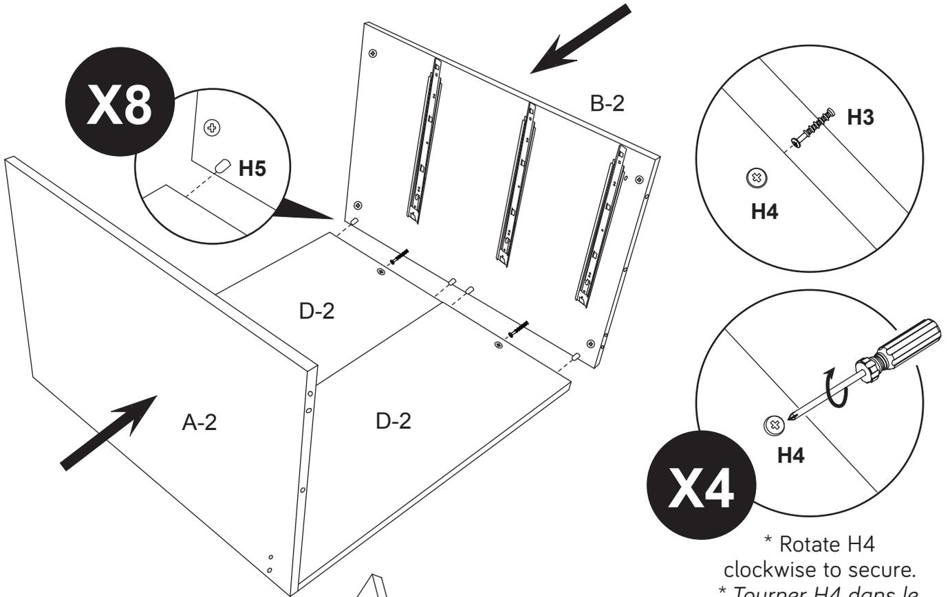
\* Rotate H4 clockwise to secure.
