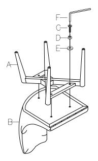
Take the Allen Key, and turn the bolts until the legs are secured. DO NOT TIGHTEN COMPLETELY. Stop when you feel you are adding force to tighten the bolt.
