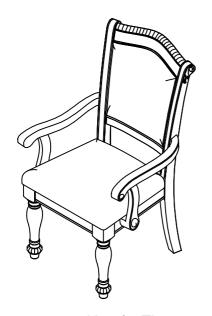
Stand chair up on an even surface and check that it is balanced. If there is a slight wobble, apply downward pressure in the corner where a leg is uneven. Keeping pressure in that corners, tighten all bolts, If balanced, apply downward pressure evenly in the center and tighten all bolts, Do not over-tighten beyond hole depth
