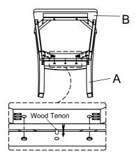
Place the Chair Back (A). Tighten the Cushion Seat(B) on the face by bolts (J)(K). Lock washer (G) and flat washer (H) with allen key (I).
