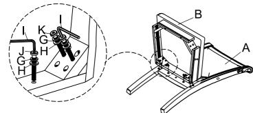
Take the Allen Key, and turn the bolts until the Mounting Plate are secure. DO NOT TIGHTEN COMPLETELY. Stop when feel you are adding force to tighten the bolt.
