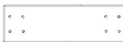
H3 MONTANT DU BANC - W4L17336 (x2) 15/16 po x 3 3/8 po x 11 po (24 x 86 x 280)
