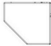
G3 SUPPORT D'ÉTAGÈRE - W4L17342 (x1) 15/16 po x 5 1/4 po x 5 7/8 po (24 x 134 x 150)
