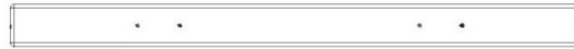
P01 POTEAU DE CLÔTURE - W4L17339 (x1) 1 7/16 po x 1 7/16 po x 19 po (36 x 36 x 483)
