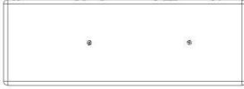
J4 PLANCHE DE SUPPORT - W4L17346 (x1) 15/16 po x 2 3/8 po x 6 11/16 po (24 x 60 x 170)
