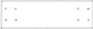
H3 MONTANT DU BANC - W4L17336 (x2) 15/16 po x 3 3/8 po x 11 po (24 x 86 x 280)
