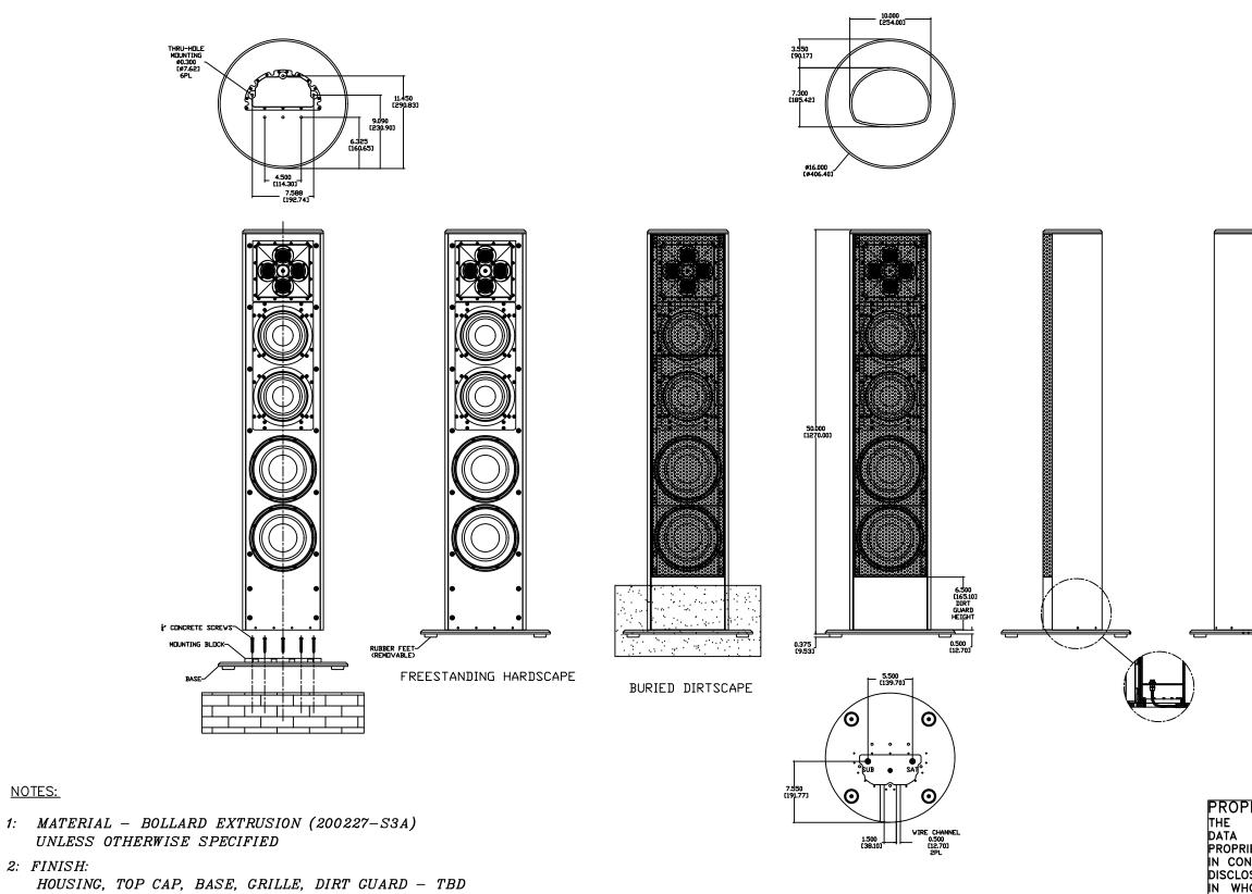
2: FINISH: HOUSING, TOP CAP, BASE, GRILLE, DIRT GUARD - TBD DRIVER RECESS, END CAP, MOUNTING BLOCK, GRILLE FRAME, DIRT GUARD FRAME, GRILLE FRAME BRACKET - STUDIO BLACK POWDER COAT UNLESS OTHERWISE SPECIFIED
