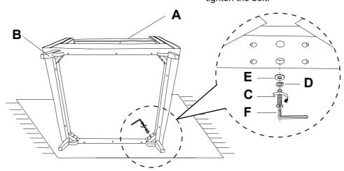
Stand chair up on an even surface and check that it is balanced. If there is a slight wobble, apply downward pressure in the corner where a leg is uneven. Keeping pressure in that corner, tighten all bolts. If balanced, apply downward pressure evenly in the center and tighten all bolts. Do not over-tighten beyond hole depth.
