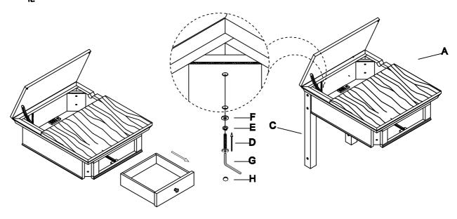
Turn Top Panel (A) down, and attach the 3rd Metal Leg (C) on it using Bolt (D), Spring Washer (E), Flat Washer (F) by Wrench (G).
