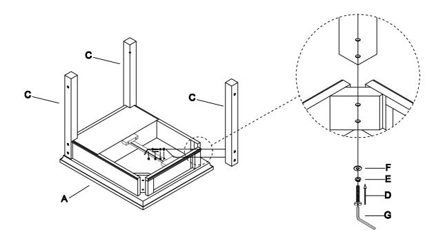
Attach the Bottom Shelf (B) onto the 3pcs Metal Leg (C) using Bolt (D), Spring Washer (E), Flat Washer (F) by Wrench (G). Then attach the 4th Metal Leg (C) to both Bottom Shelf (B) and Top Panel (A) by the same method. Finally lock them up to 100%.
