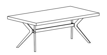
This page lists all the contents included in the box. Please take the time to identify the hardware as well as the individual components to this product. As you unpack and prepare for assembly, place the contents on a carpeted or padded area to protect them from damage. Attach Leg (B) to bottom of Table Top (A) using Bolt (E), Spring Washer (G), Flat Washer (H) with Allen Key (I).
