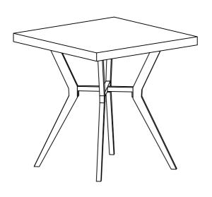
This page lists all the contents included in the box. Please take the time to identify the hardware as well as the individual components to this product. As you unpack and prepare for assembly, place the contents on a carpeted or padded area to protect them from damage. Attach Leg (B) to bottom of Table Top (A) using Bolt (D), Spring Washer (E), Flat Washer (F) with Allen Key (G).
