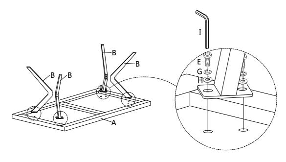
Attach Iron (D) to Leg (B) using Bolt (F), Spring Washer (G), Flat Washer (H) with Wrench (J).
