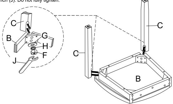
Take the Wrench, and turn the bolts until the legs are secure. DO NOT TIGHTEN COMPLETELY.
