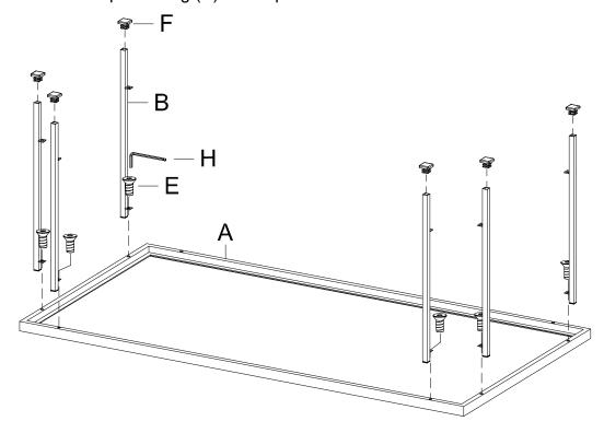
Attach the Marble Pattern Bottom (C) to the Leg (B) using Bolt (E) with the Allen Wrench (H).
