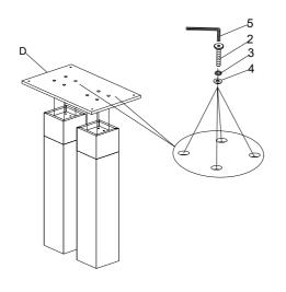
STEP 4: Assembly table legs (B) and link board (D) with the table top (A)
