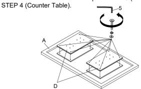
STEP 3: Assembly table legs (B) and link board (D) with the table top (A)
