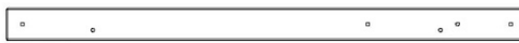
H4 | LISSE DE PLANCHER - W4L14934 (x1) | 1 po x 3 3/8 po x 54 7/8 po (24 x 86 x 1 394)
