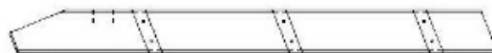
H79 | MONTANT GAUCHE - W4L14944 (x1) | 1 po x 3 3/8 po x 38 3/8 po (24 x 86 x 976)
