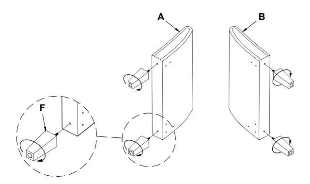
2 Attach Arm Frame - Left & Right (A & B) to Back Cushion (C) using JCBC Bolt (H), Spring Washer (K) and Flat Washer (J) with Allen Key (M).
