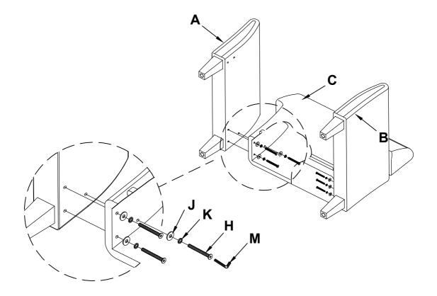
**3** Attach Stretcher (D) on Arm Frame - Left & Right (A & B) using JCBC Bolt (I), Spring Washer (K) and Flat Washer (J) with Allen Key (M).
