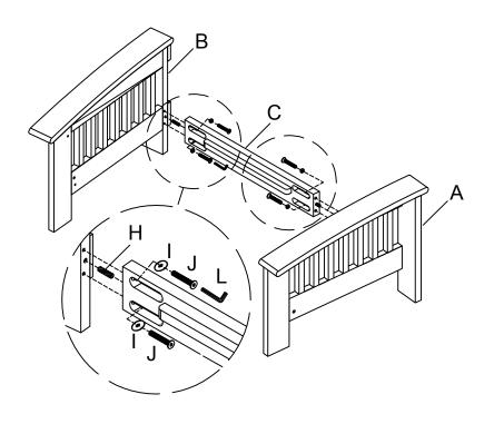
Insert Wood Dowel (H) into the middle holes of the Back Panel (D). Then, attach the Back Panel (D) to the Arm Frame-Left & Right (A & B) using JCBC Bolt (J) with Allen Key (L).
