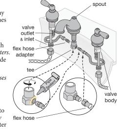
• Check for leaks if only replacing faucet and drain is already installed by first turning faucet handles to the OFF position and then turn water supply valves ON.
