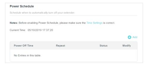
4. Specify a time period in the Power-Off Time field and days for the power-off to repeat, and the extender will be off during this period in the days you specify.
