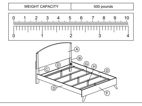
STEP 1: Assemble the Headboard Cross Bar (D) between the Headboard RSF Leg (B) and Headboard LSF Leg (C) by using the Allen Key (6) and the hardware Long Bolt 1/4" x 2" (2) & Spring washer (3).
