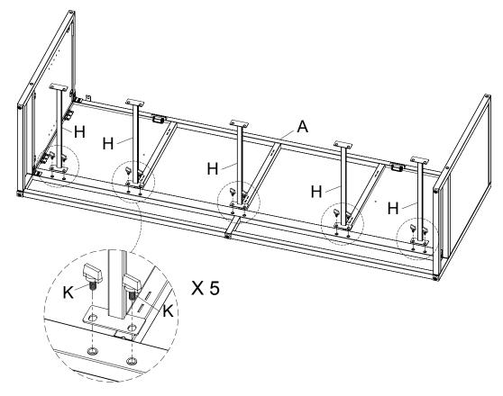
6 Attach the Back Frame (B) to the Front Frame (A) and Cross Bar (H) by using Bolt (K) as shown.
