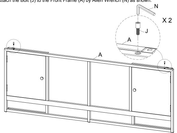
Attach the Bolt (J) to the Front Frame (A) by Allen Wrench (N) as shown.
