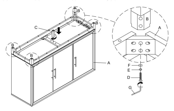
2 Adjust the levelers at the bottom of the Leg (B & C) to keep the Server leveled.
