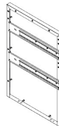
S4 LEFT CABINET SIDE PANEL ASSEMBLY R - A4M04465 (x1) 35 1/4"x23 11/16"x1 7/8" (48.3x601.5x896)
