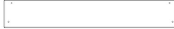
L2 | PLANCHE DE SOL DU NID DE CORBEAU - W4L13304 (2) | 5/8"x4 3/8"x27" (16x112x686)
