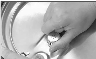
8. Remove the float valve seal (1) while supporting the float valve from the other side of the lid. Then remove the float valve (2).
