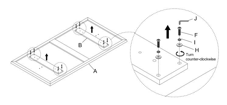
Attach the Mounting Plate (B) to the Leg (C) by inserting Dowel (K), and using Allen Bolt (F), Lock Washer (I) and Flat Washer (H) with Allen Key (J).
