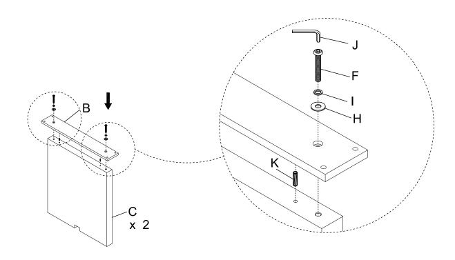
Attach the Mounting Plate (B) to the Table Top (A) using Allen Bolt (F), Lock Washer (I) and Flat Washer (H) with Allen Key (J).
