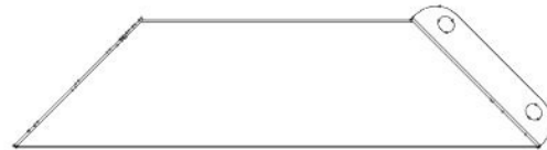
C02 ASSEMBLAGE DE CORBEAU - A4M03526 (x1) 21 13/16"x5 1/4"x2 3/4" (70x134x553.5)
