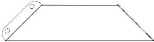
C01 ASSEMBLAGE DE CORBEAU-A4M03525 (x1) 2113/16"x5 1/4"x2 3/4" (70x134x553.5)
