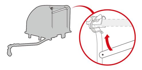
Insert the part C handlebar into the trailer. Press the buttons on the sides of the handlebar to adjust it to your desired position. Compress the metal pins while inserting the handlebar to lock it in place.
