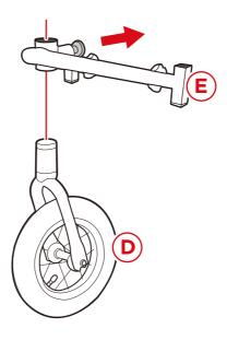
2 Loosen the two back knobs on the part E fork, slide the fork/wheel onto the front of the trailer, and then tighten the knobs.
