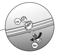
Remove PB1 ( $1/4 \times 3/4$ " Pan Bolt), The bolt (PB1) will no longer be needed, but keep the lock nut (LN1)
