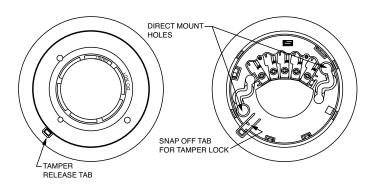
Figure 1: Tamper-Resistant Feature/Wiring
