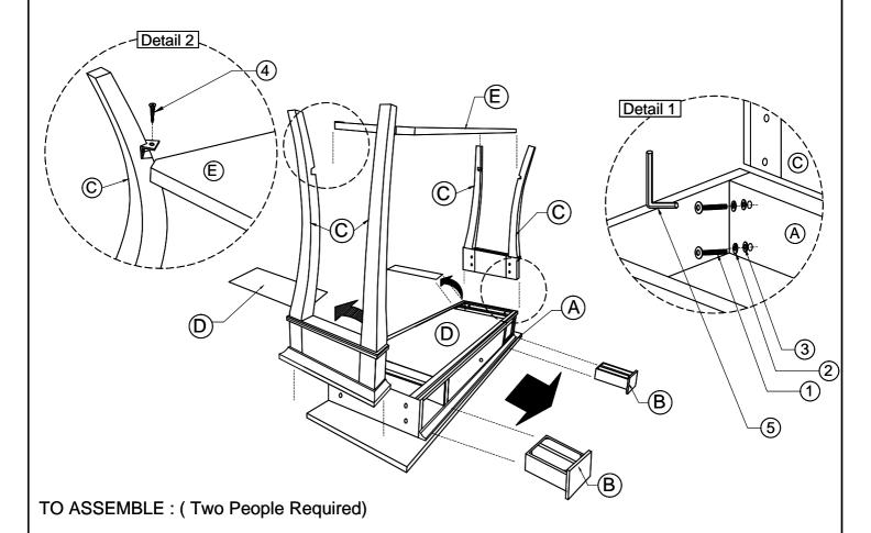
Step 1: Remove Drawers (B) and turn the table (A) upside down on a soft, clean surface
