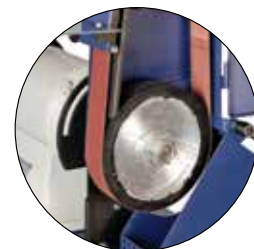
Easy toolless belt changes with swing away belt guarding
