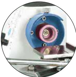
Cup wheel Self-trimming Runs dry
