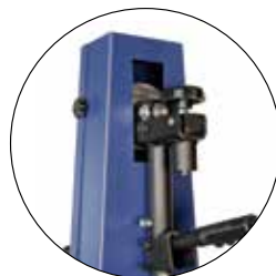
Simple belt tension and belt tracking systems
